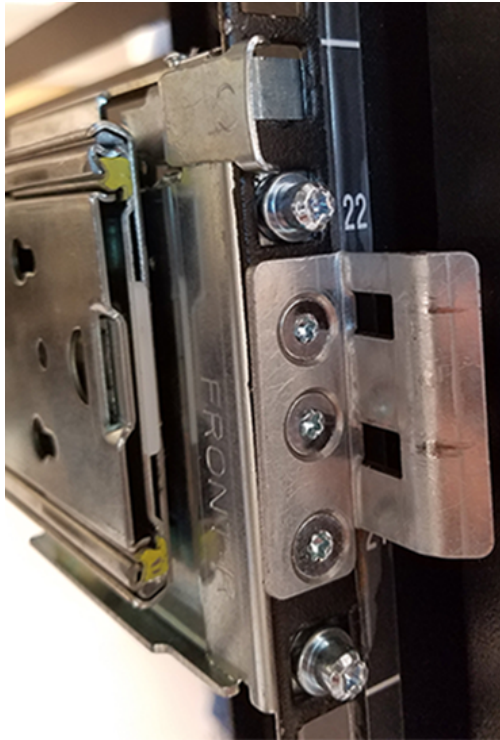
Figure 116: Rack Latch Bracket Installed
