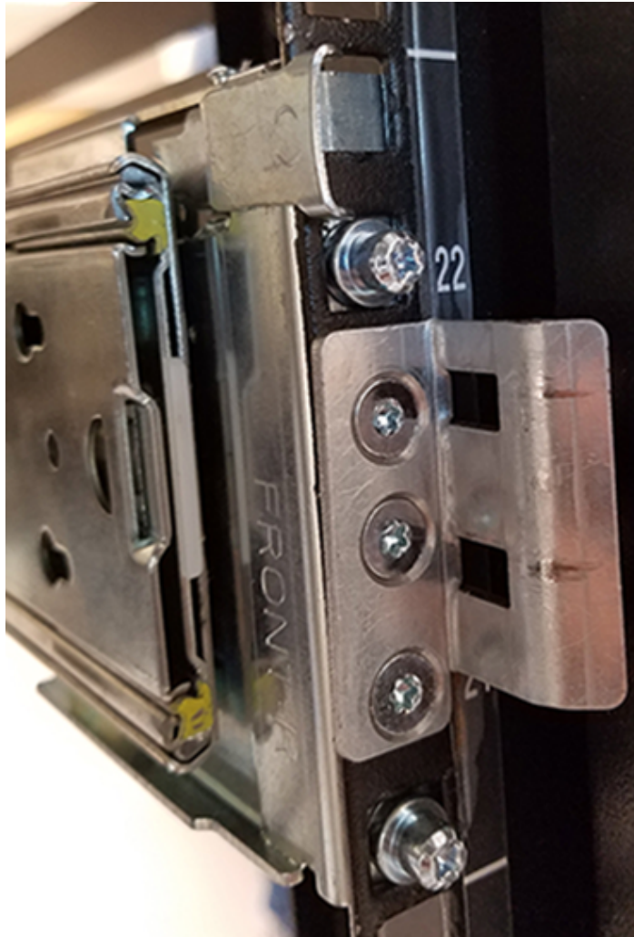
Figure 127: Rack Latch Bracket Installed
