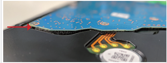
This is a photo WITH insulator (normal state)
