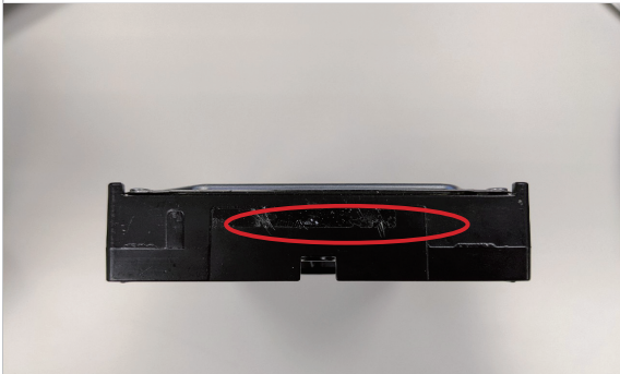
Missing module label
