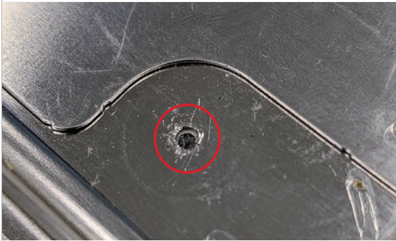
Damaged air filter
