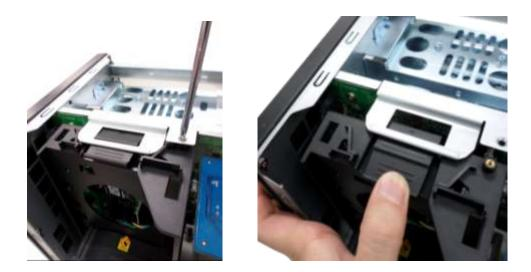
4. Pull the retention clips on each side so that the module can be removed. Remove the installed memory modules.
