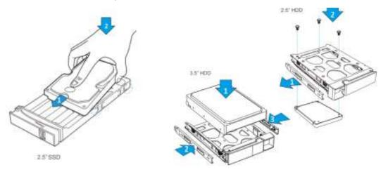
3. Insert the hard drive trays into the NAS all the way to the rear and push the lever back until you hear a click then pull up the tray lock to ensure the tray is completely fixed in the system.
