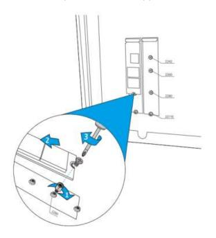
4. Reinstall the fan module and fasten its screw, reconnect the cable, put the cover back and fasten all the screws.
