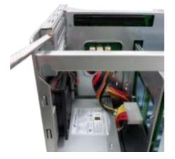
ii. Grasp the edge of the graphics card. Align the notch on the gold edge of the card with the notch in the PCIe slot. Insert the graphics card into the PCIe slot until it cannot go any further.
