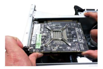
iii. Fasten the screws to completely fix the graphic card.
