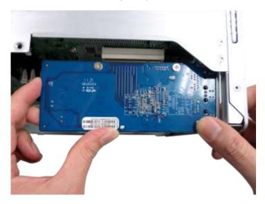
iii. Fasten the screw to keep the expansion.
