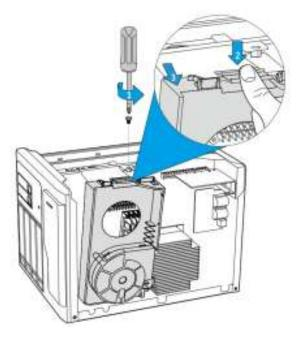
3. The TVS-x82 series has two M.2 SSD slots and supports 4 different M.2 SSD sizes (2242, 2260, 2280 and 22110). Move and fasten the riser screw to the appropriate position according to your M.2 SSD size. Then insert the M.2 SSD to the slot and secure it in place with the supplied screws.
