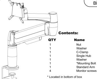
Required Tools: 6mm Allen wrench 17mm Deep socket
