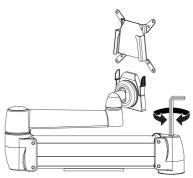
Position Arm so it is parallel to desk surface. Turn bolt wise for lighter monitors.
