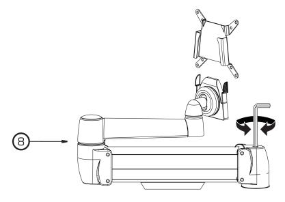
Position Arm so it is parallel to desk surface. Turn bolt clock wise for lighter monitors.
