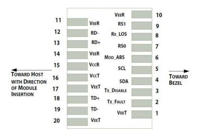
Pin-out of connector Block on Host board
