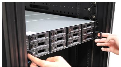
2 With the help of another person, carefully remove the chassis from the rack. Then, slide the inner rail attached to the chassis toward the front panel of the chassis to detach it.
