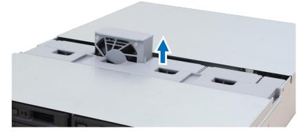
**5** Prepare a new fan and slide it into the your RS3621RPxs. Make sure that the fan is aligned properly, as shown below.
