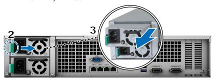
4 Prepare a new PSU. Insert it into the empty slot until you hear a click.
