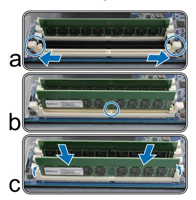
Note: Hold the memory module by its edges and avoid touching the gold connectors.
