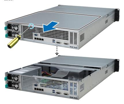
**Note:** When you remove the rear top cover, sensitive internal components are exposed. Avoid touching anything other than the memory assembly when removing or adding memory.
