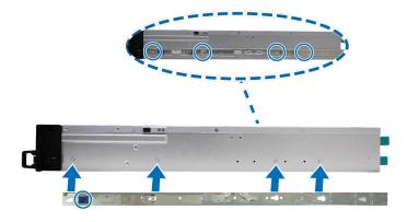
4 With the help of another person, carefully align the inner rail to the outer rail assembly.
