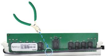
**Note:** Avoid touching any components on the motherboard when cutting the cable tie.
